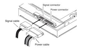
Figure 2. Attaching SATA cabling
